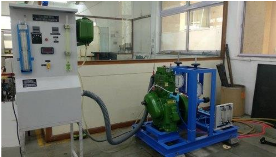
Figure 3.3: IC Diesel engine test set-up
