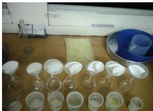
Figure 3.4. Extraction of samples for aflatoxin analysis.
