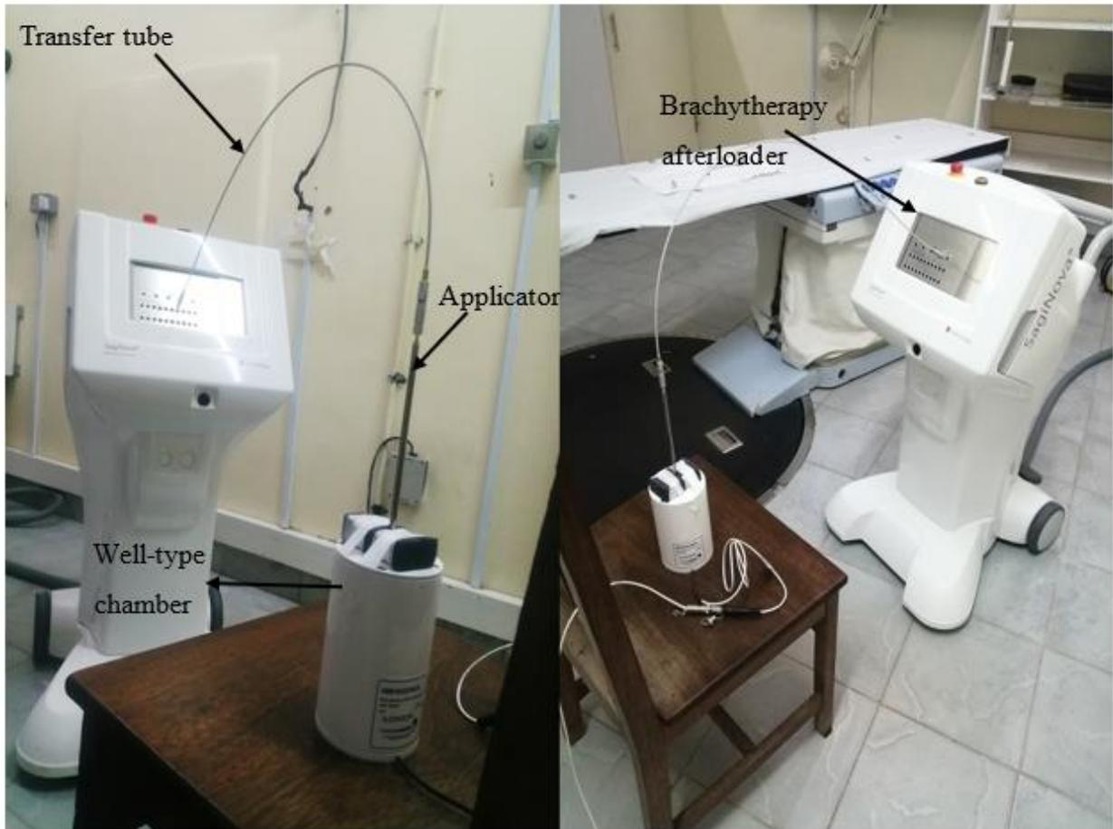
**Figure 3.5:** The measurement set up in the bunker.
