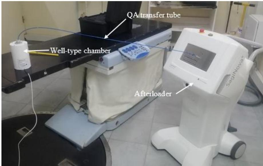
**Figure 4.1:** Dwell position sensitivity measurements setup.
