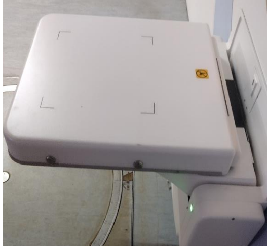
Figure 3. 8. Closer view of the EPID
